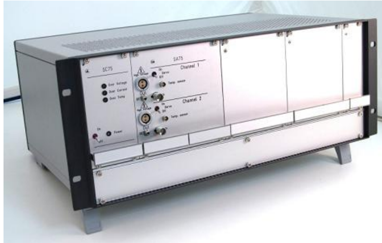
Figure 7: SA75D assembled in standard 19 inches rack.
