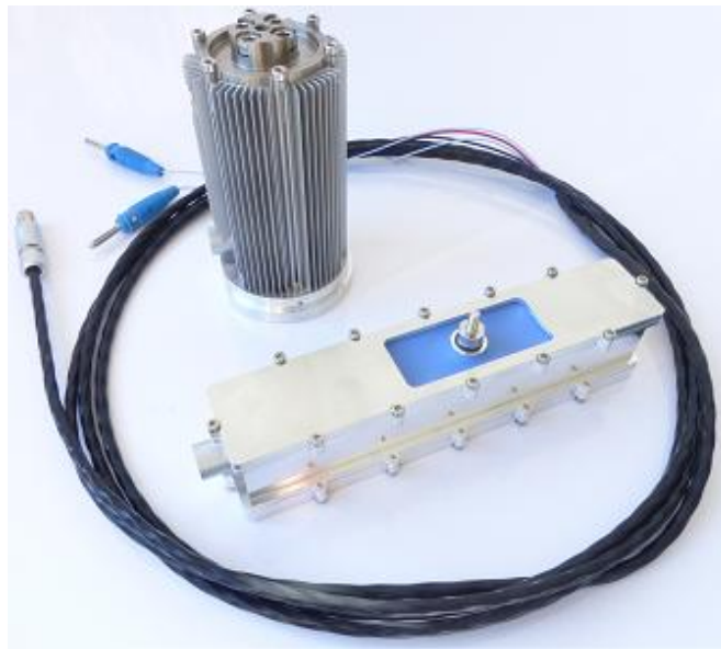
Figure 9: Encapsulated PPA80L and APA2000L.
